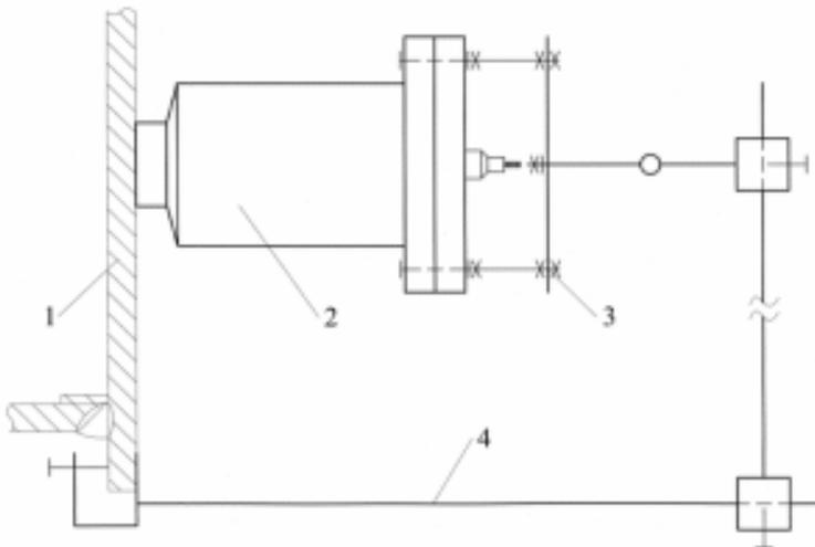
*Fig.1. Diagram of mounting the portable electrochemical device to the investigated section of the crane with a hinge suspension:*
