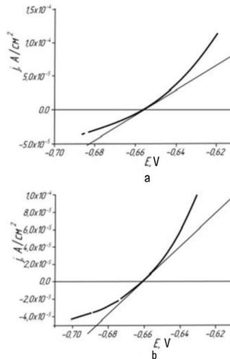
Fig. 9. Polarization curves of crane steel in 0,3% NaCl solution:
