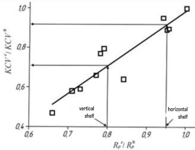
Fig. 8. Correlation between relative changes (the ratio of the impact toughness of the used material  $KCV^e$  to the impact toughness in the initial state  $KCV^0$ ) and polarization resistance (the ratio of the polarization resistance of the used material  $R_p^e$  to the polarization resistance of the steel in the initial state  $R_p^0$ ) of different crane components. The arrows indicate the values of  $R_p^e$  determined on crane
