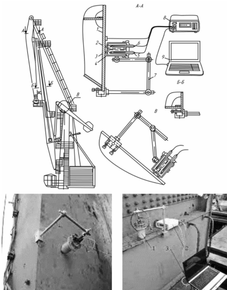
*Fig. 5. Examples of mounting the electrochemical device to the metal structure of the crane*
