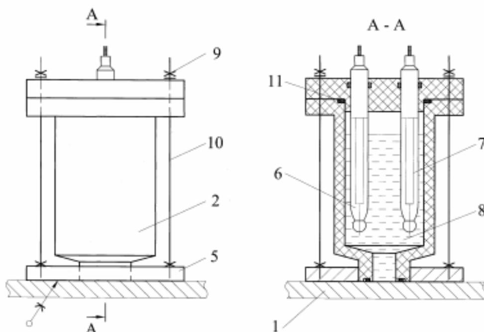
*Fig. 2. Diagram of the portable electrochemical device mounted to the investigated section of the crane with a mounting washer:*
