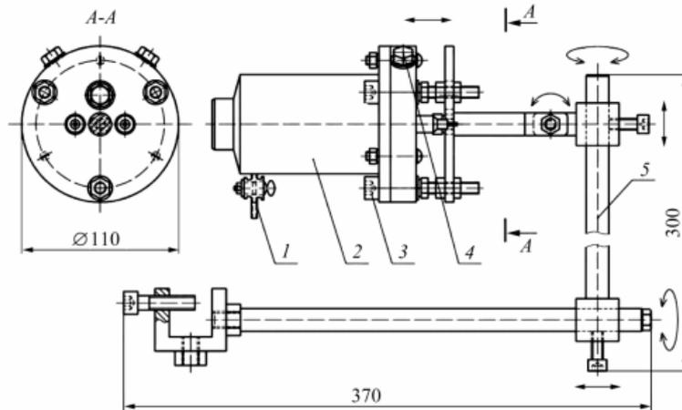
Fig. 3. Example of mounting a portable three-electrode electrochemical device:
