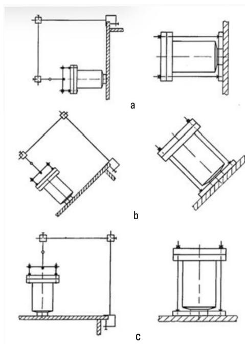
*Fig.6. Mounting options of the ECP to the investigated section of the metal crane structure:*
