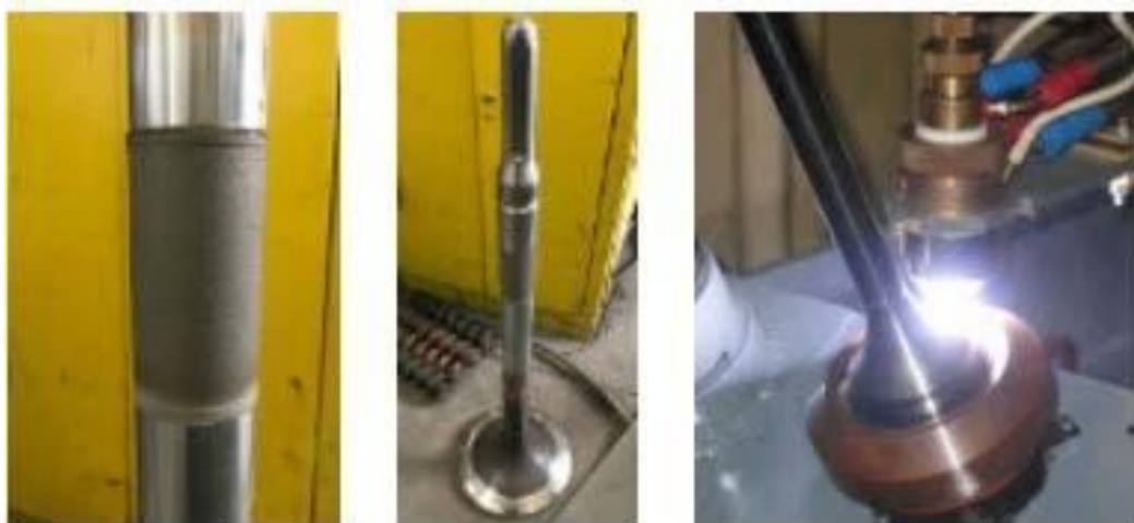
Fig. 2. Plasma surfacing with self – fluxing powder containing exothermic flux
